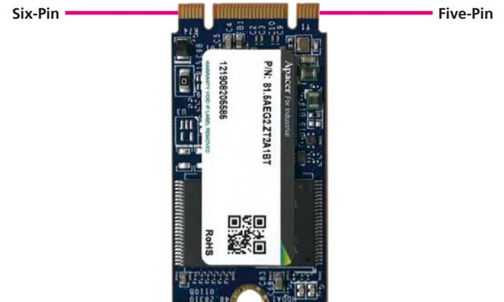
3. Insert the M.2 module into the M.2 slot at 45-degree angle until the gold-plated connector on the edge of the module completely disappears into the slot.
