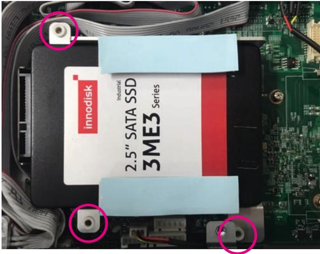
4. Secure the internal storage bracket with screws.
