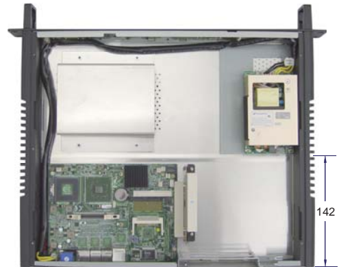
19" 1U fanless system ( CI945A / 963A ) with internal PSU 150W * PCI Card length: 142 mm
